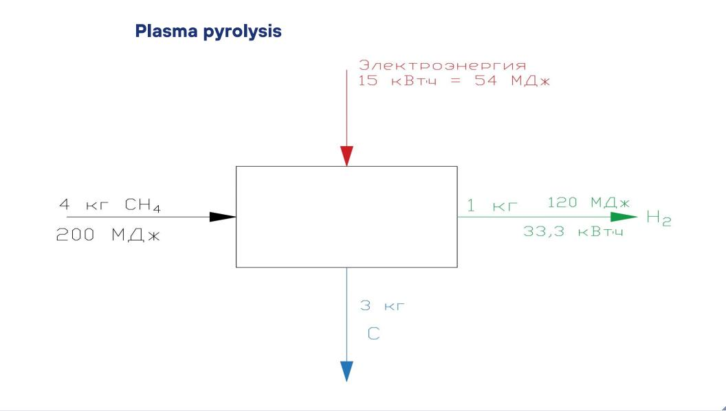
Basing by the above analysis, hydrogen obtained by electrolysis of water has a higher energy value than hydrogen obtained by plasma pyrolysis.
