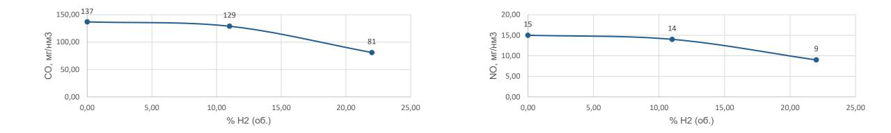
The values of concentrations of carbon monoxide (CO) and nitrogen oxides in the flue gases of the boiler are given with an excess air coefficient equal to one.
