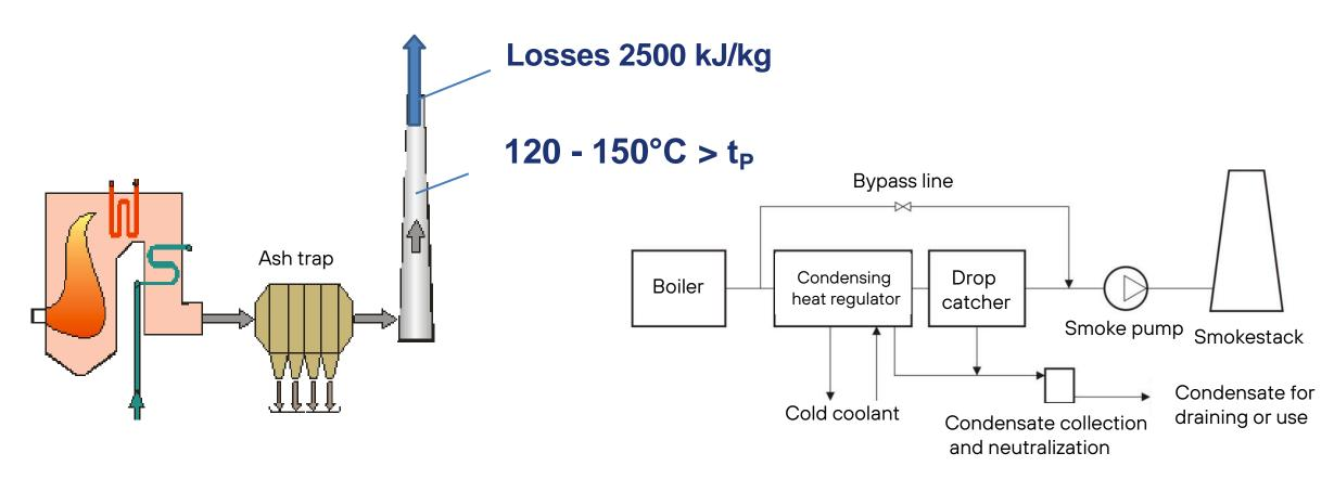
Water vapor, like carbon dioxide, is a greenhouse gas. Reducing its emissions into the atmosphere is also an urgent task. Simultaneous reduction of water vapor and carbon dioxide emissions into the atmosphere during natural gas combustion is possible due to condensation of flue gas water vapor before their release into the atmospheric air.
